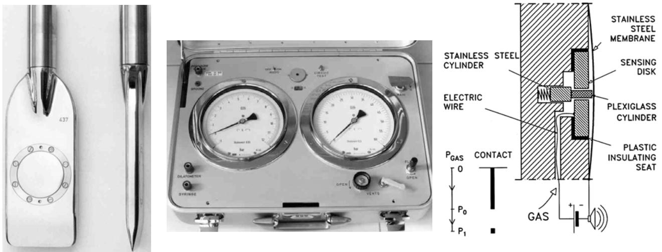
Figure 8. Marchetti dilatometer (DMT): front and side view of the ‘blade’ (left); view of the readout unit (centre); and schematic of the measuring system for determining ‘liftoff’ and displacement of 1 mm (right).
