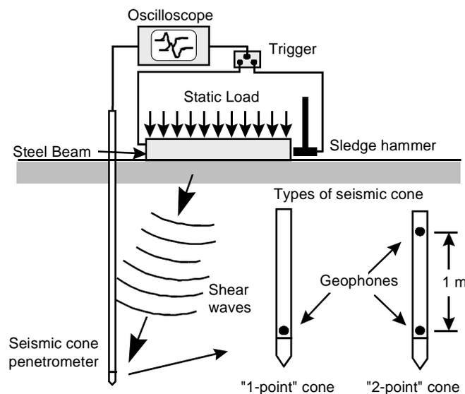
Figure 9: Schematic layout for seismic CPT test.
