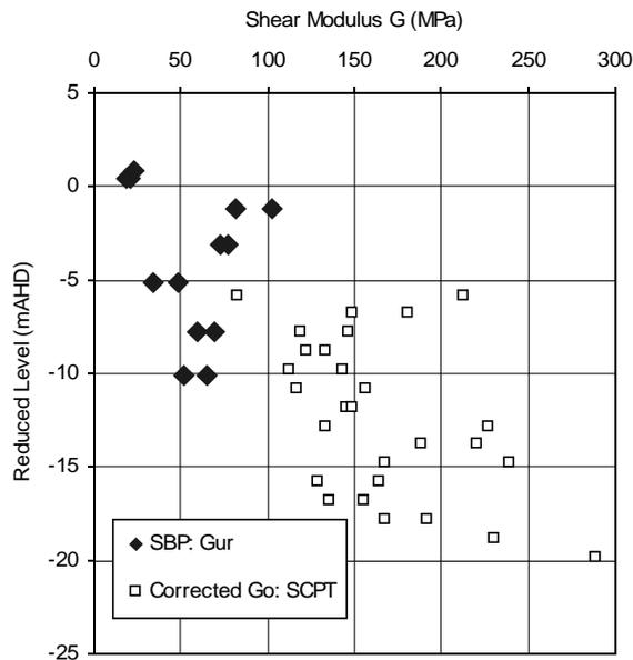
Figure 20. Comparison of corrected  $G_0$  values inferred from SCPT data and SBPT  $G_{ur}$  data at Site M (SCPT  $G_0$  values from Figure 19(a) corrected for stress level change due to excavation at site).
