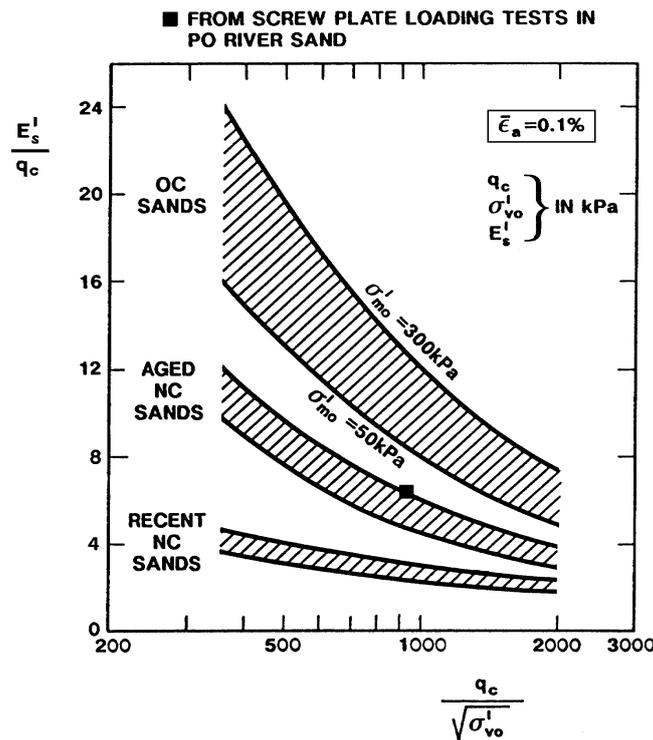
Figure 6: Ratio of ‘working strain’ stiffness  $E'_s$  to  $q_c$  versus  $q_c/\sqrt{\sigma'_{vo}}$  for sands with different stress histories (Baldi *et al.*, 1989).
