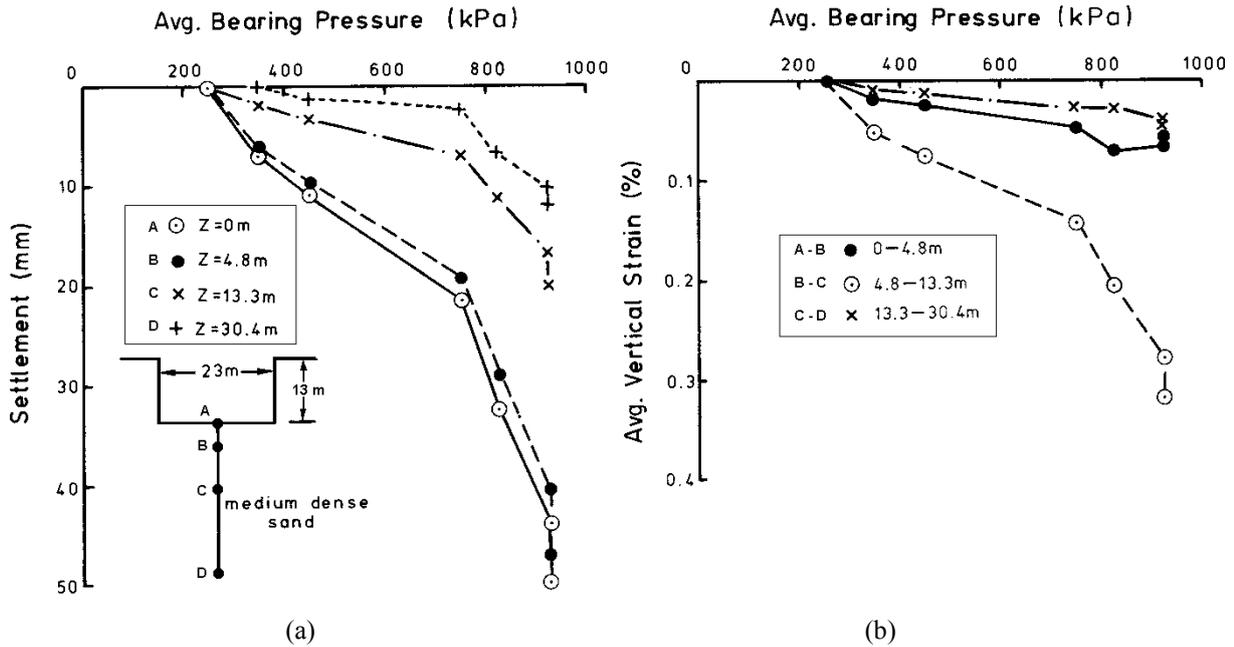
Figure 4: (a) Settlements at various depths beneath the foundation raft for a tall hotel in medium dense sand in Berlin; and (b) corresponding vertical strains in the ground for the same case (after Burland, 1989).
