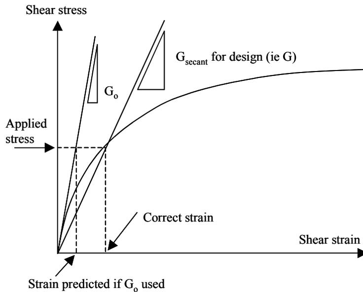
Figure 1: Illustration of non-linear stiffness of soil, and definition of initial tangent shear modulus (or small strain).
