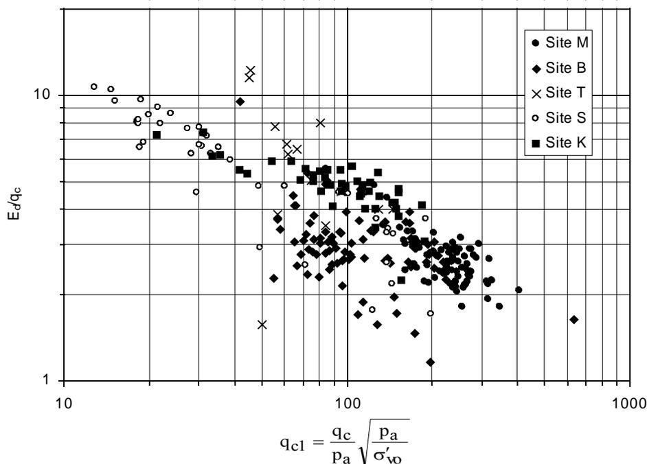
Figure 23: Relationship between the dilatometer modulus,  $E_d$ , and  $q_c$  observed in Perth CBD.
