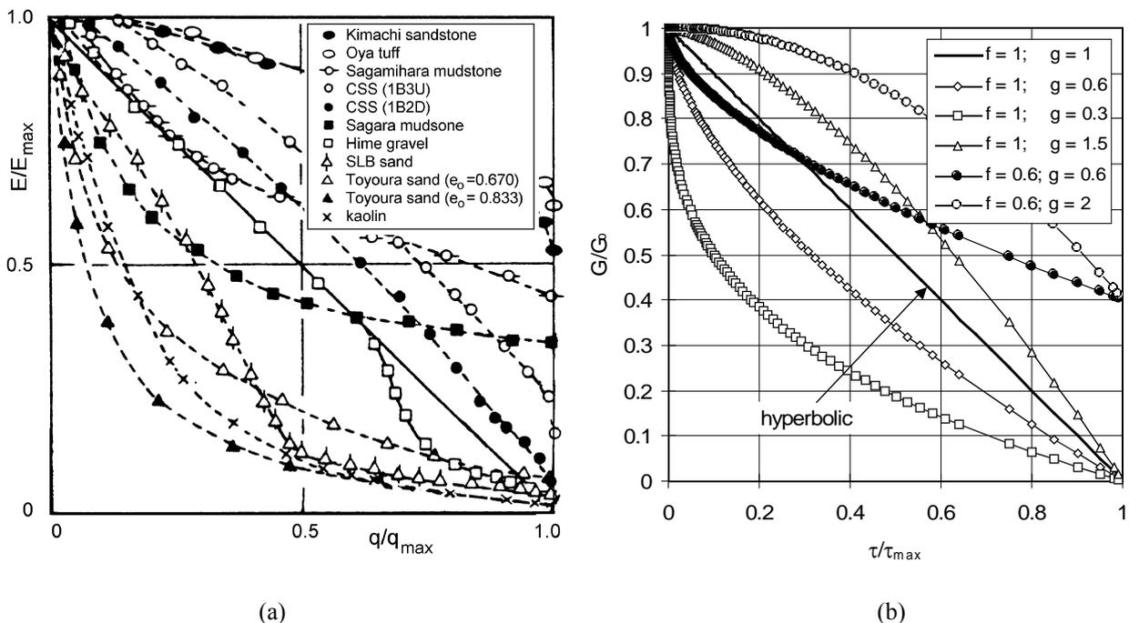
Figure 3: Stiffness degradation plotted as normalised stiffness versus normalised mobilised shear stress: (a) data from various soils and soft rocks after Tatsuoka and Shibuya (1991); and (b) shapes of curves obtained using the ‘distorted hyperbolic’ model of Fahey and Carter (1993).
