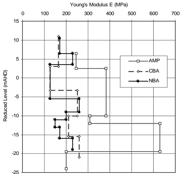
Figure 17: Stiffness profiles back-analysed for the AMP, CBA and NBA buildings (data from Fraser, 1975).
