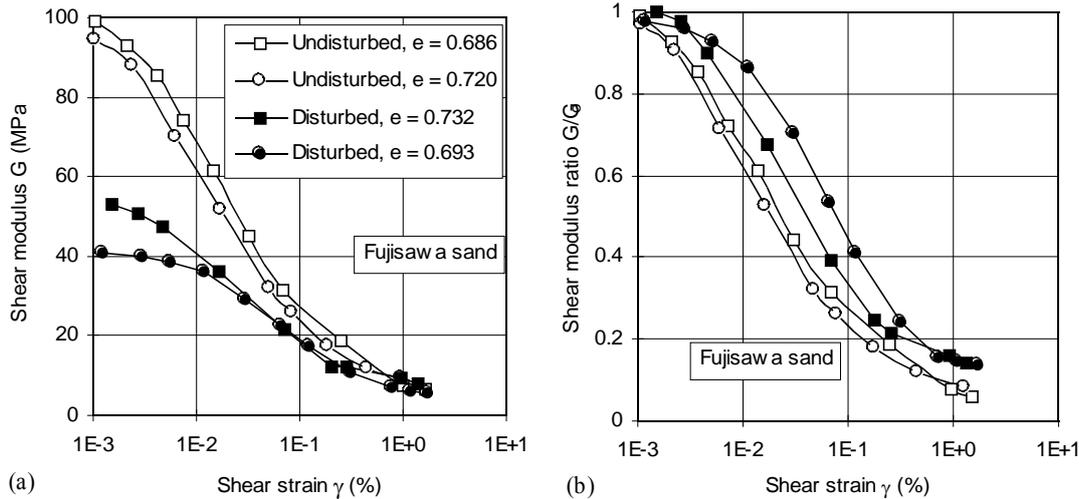
Figure 2: Modulus degradation curves for Fujisawa sand plotted as (a) G versus  $\gamma$ , and (b)  $G/G_0$  versus  $\gamma$  (replotted from Ishihara, 1996).
