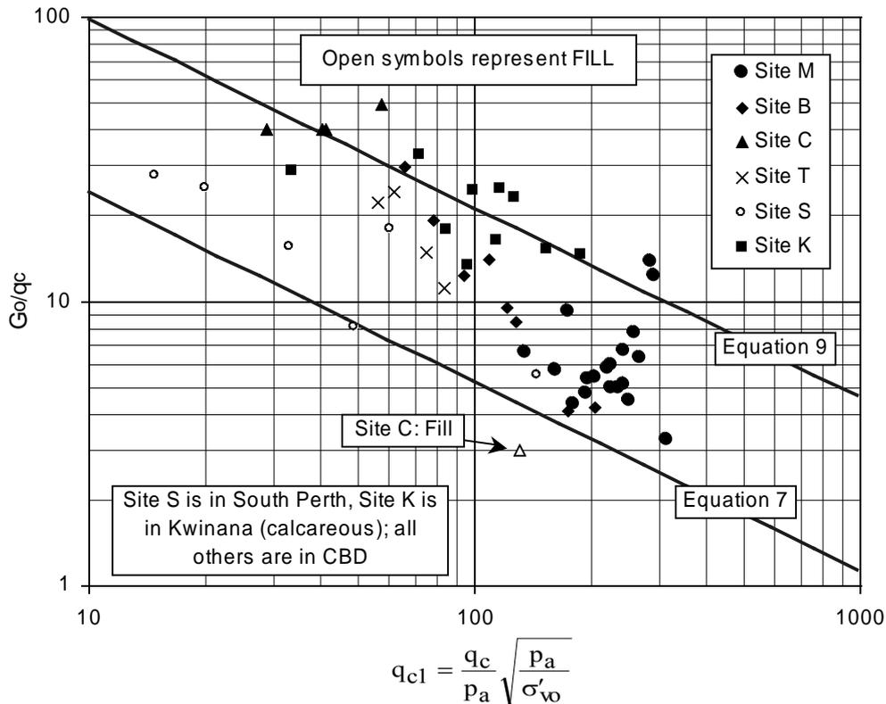
Figure 22: Relationship between  $G_0$  (from SCPTs) and  $q_c$  observed in Perth CBD sand.
