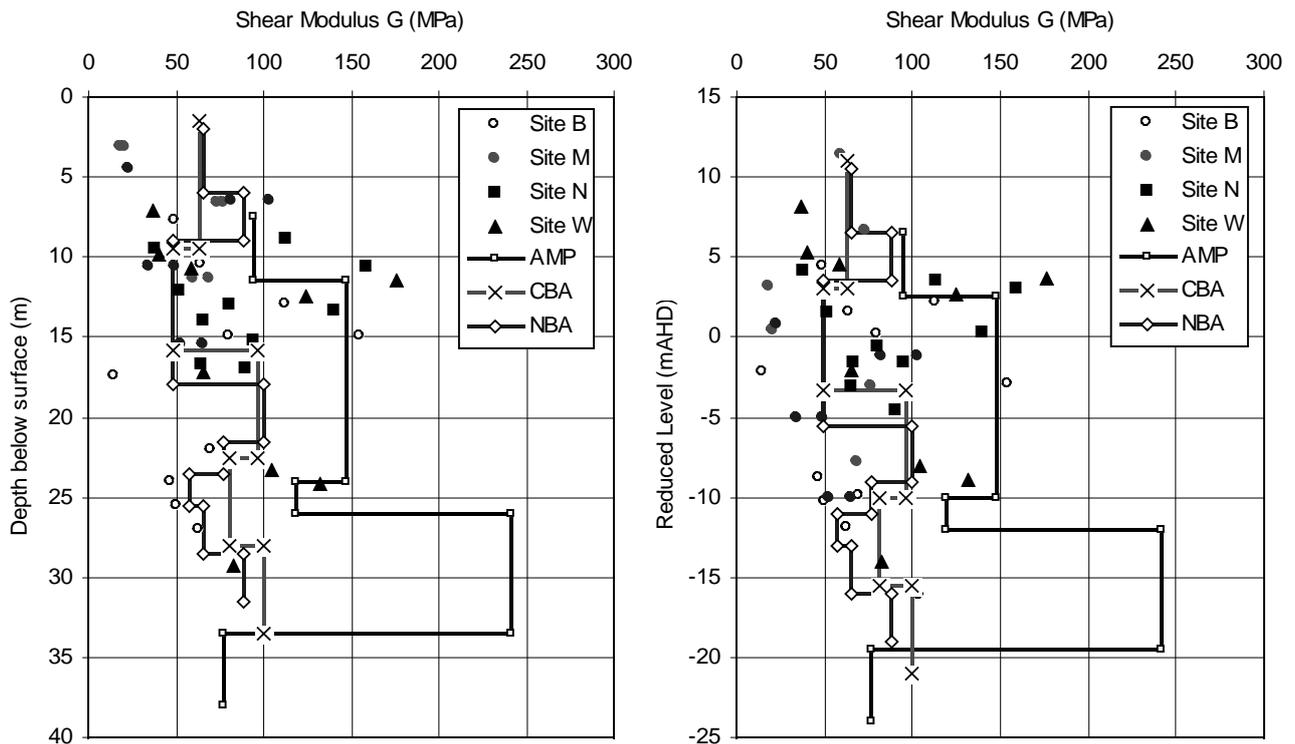
Figure 18: Shear modulus ( $G_{ur}$ ) profiles from SBP tests at various sites in the CBD, compared to  $G$  values deduced from the  $E$  values from Figure 17 (assuming Poisson’s Ratio  $\nu = 0.3$ ).
