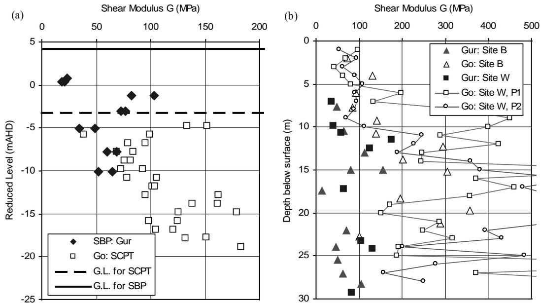
Figure 19: Seismic CPT  $G_0$  values compared to SBP  $G_{ur}$  values: (a) Site M (note excavation at site after SBP tests but before SCPT tests); and (b) Site B and Site W.
