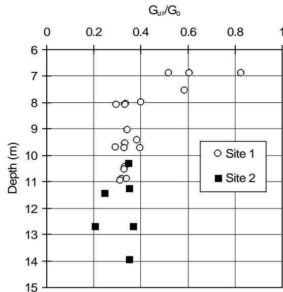
Figure 11: Ratios of  $G_{ur}$  from SBP tests and  $G_o$  from SCPT test at two sites in Perth (not in the CBD) plotted against depth (Fahey, 1998). The sand at Site 1 is of the Spearwood Dune System, and that at Site 2 is Bassendean Sand.
