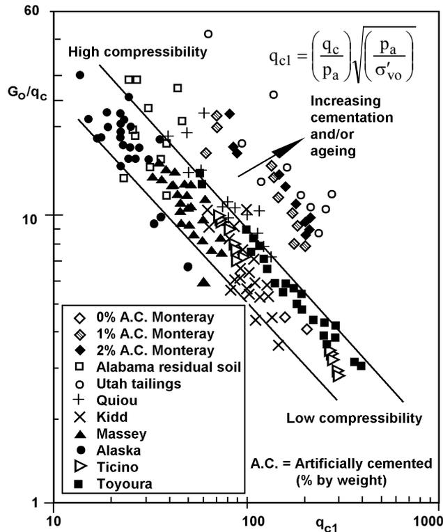
Figure 10: Plot of  $G_0/q_c$  versus  $q_{c1}$  for various sands (after Robertson, 1997, scanned and re-plotted).
