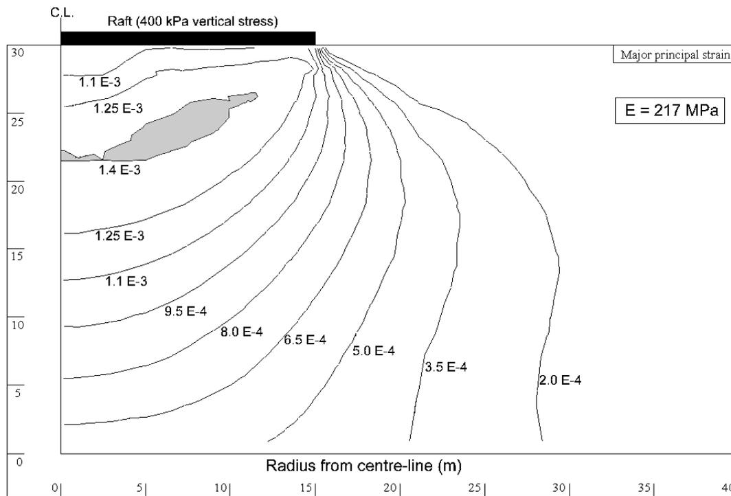
Figure 5: Contours of major principal strains under a flexible raft, 30 m in diameter, resting on a 30 m deep layer of elastic soil, with  $E = 217 \text{ MPa}$ , and  $\nu = 0.3$ .
