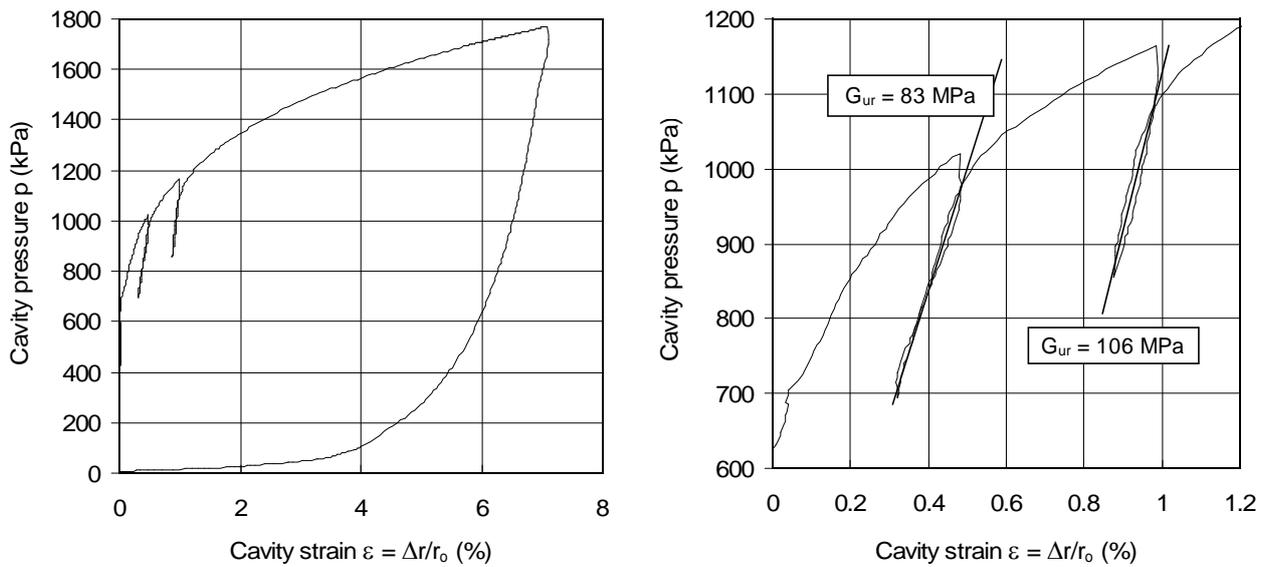
Figure 7: Results of SBP test in stiff clay layer at depth of 29.5 m, at the western end of CBD. The plot on the right shows an expanded version of the one on the left.
