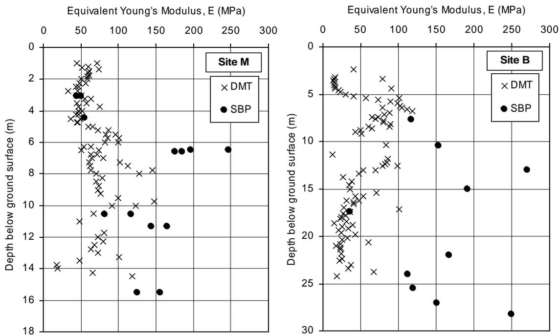
Figure 21: Equivalent Young's Moduli derived from DMT results and from SBPT  $G_{ur}$  data at Site M and Site B.
