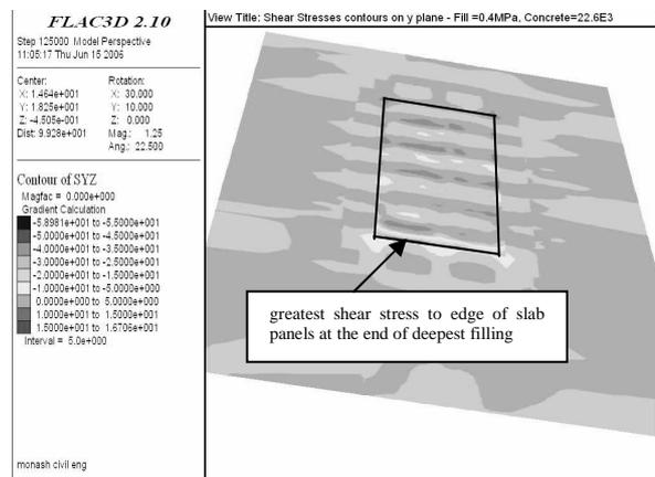
Figure 12: Contours of Y plane shear corresponding to maximum deflection ( $\Theta$ )
