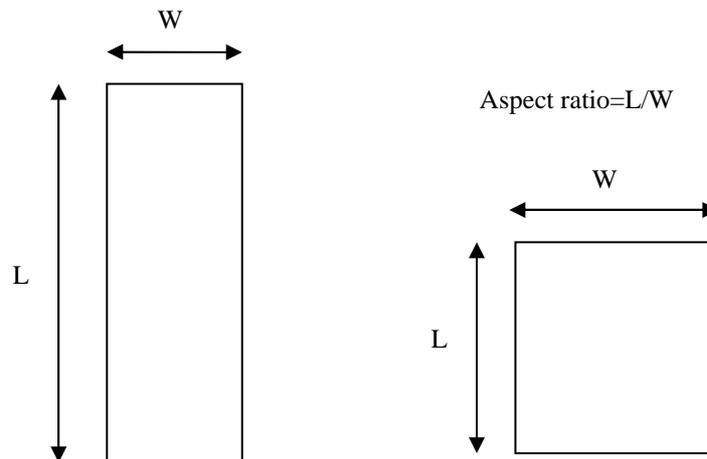
Figure 8: Definition of aspect ratio.
