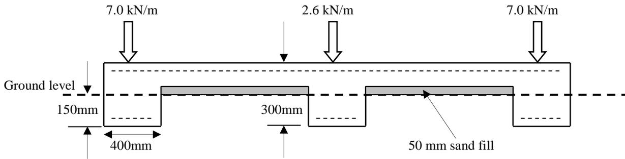
Figure 2: Raft footing cross section.
