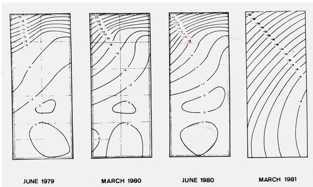
Figure 3: Surface settlement of a raft footing (in mm) on NEF at Chelsea Site (Holland, 1978).
