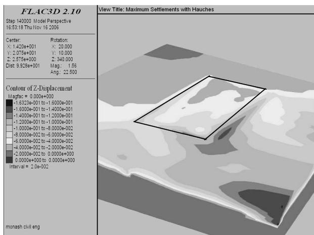
Figure 13: Settlement in footing with haunches throughout.
