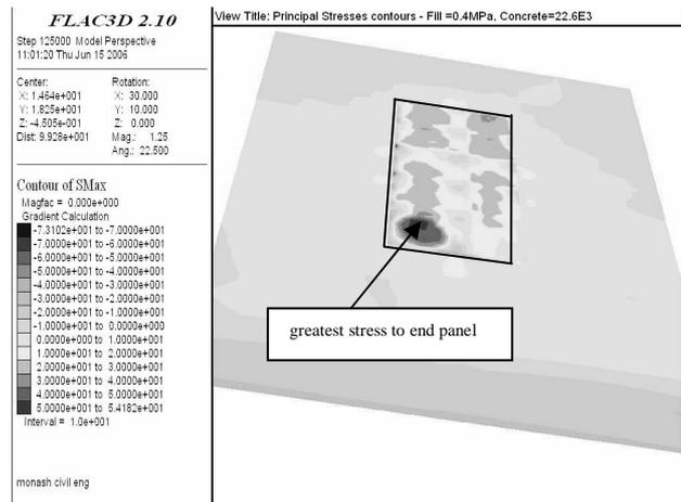
Figure 10: Contours of principal stresses corresponding to maximum deflection ( $\Theta$ ).
