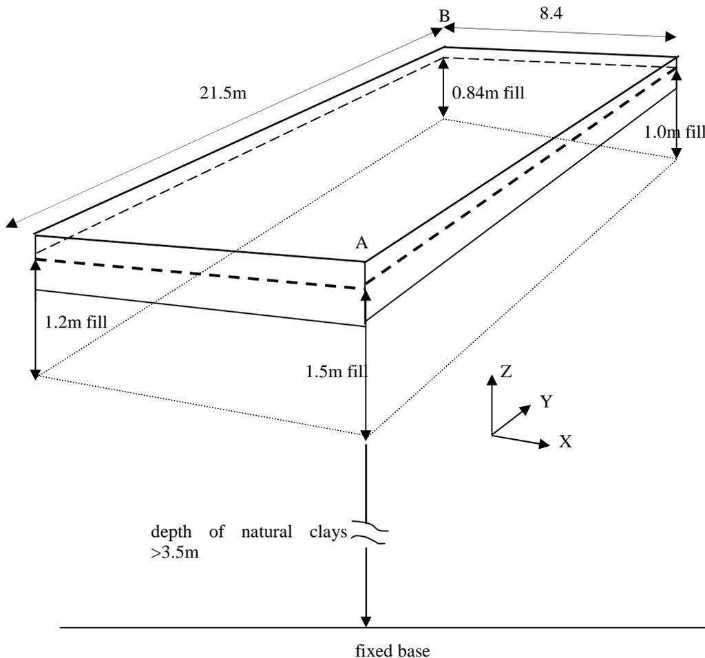
Figure 6: Simplified soil-raft model.
