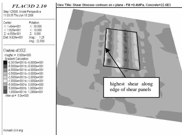
Figure 11: Contours of X plane shear corresponding to maximum deflection ( $\Theta$ )
