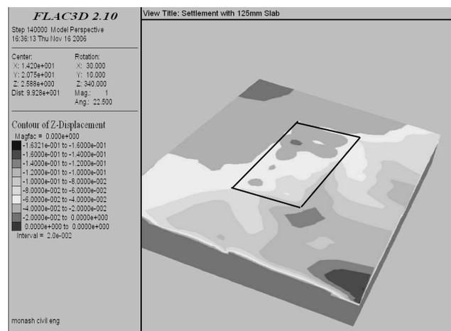
Figure 14: Settlement in footing with 125 mm slab panels throughout.
