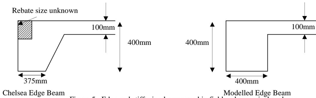
Figure 5: Edge and stiffening beams used in field and numerical analyses.
