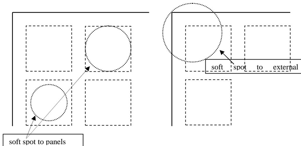
Figure 1: Critical soft spot locations (Holland, 1978).
