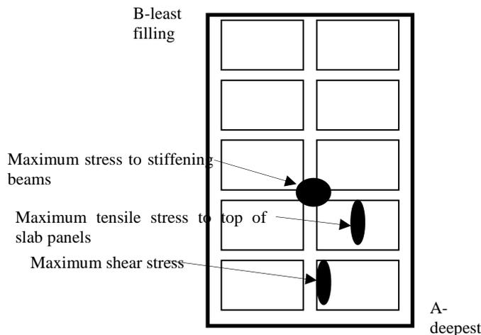
Figure 7: Finite element model – maximum stress locations (not to scale).
