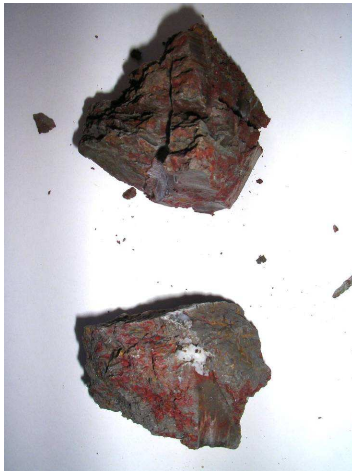
Figure 10a: Comparison of virtually identical dark grey/red mottled clays from the Lambeth Group (top), Guildford Formation (bottom).
