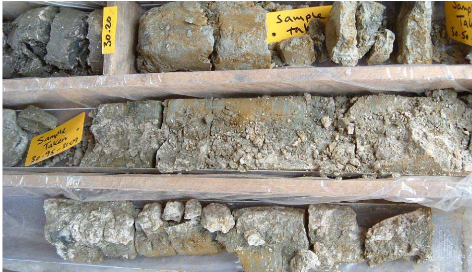
Figure 5: Hard beds. Calcretes in a Crossrail cored borehole in east London. (Lower Mottled Beds, Reading Formation).
