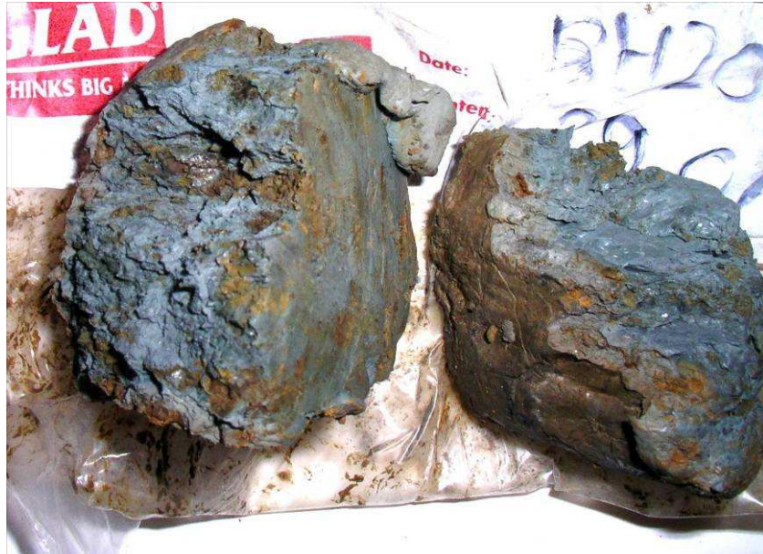
Figure 10: Blue and brown mottled clays/silts, Guildford Formation.
