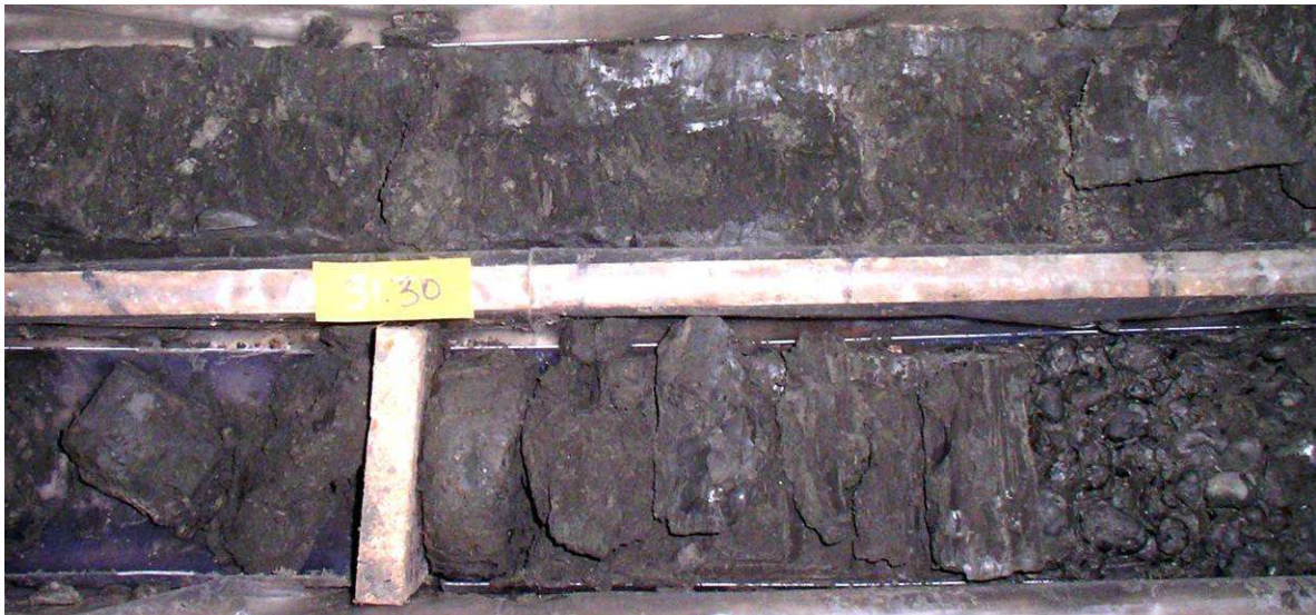
Figure 2: Laminated shallow marine to estuarine sediments of the Upnor Formation. Rotary core from King's Cross, north London.
