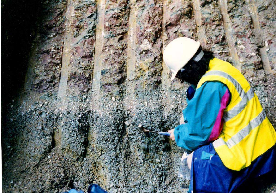
Figure 3: Upnor Formation/Lower Mottled Beds Pebble Beds – Canada Water Station excavation, Jubilee Line Extension Project.
