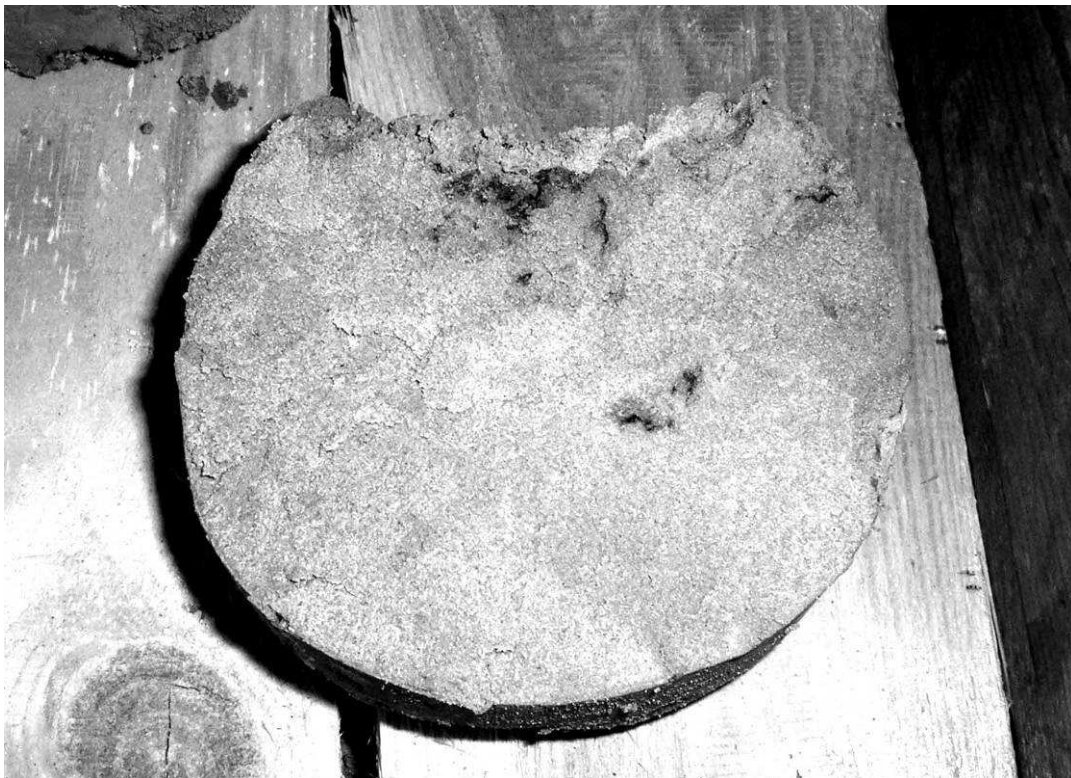
Figure 7a: Organic channel sands in Laminated Beds, Woolwich Formation, from borehole for Thames Water Ring Main Extension project, Brixton, south London. Grey sand shows black fossil root remains.
