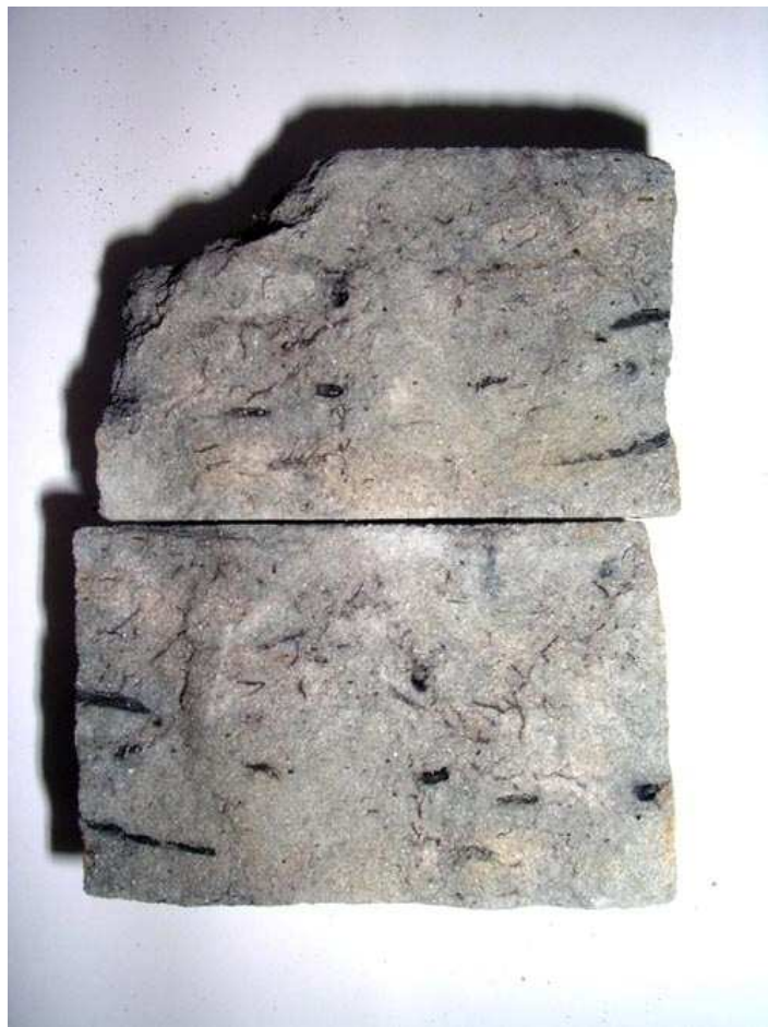
Figure 12: Organic channel sands, Guildford Formation. As in the Lambeth Group the black areas are fossil roots.
