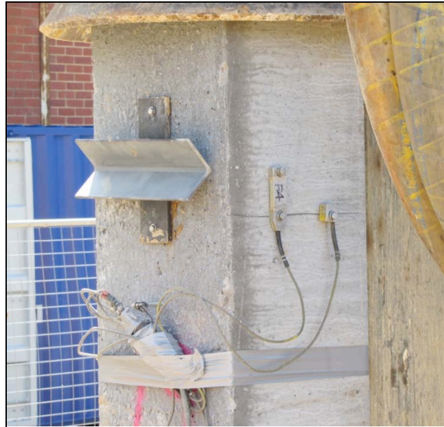
Figure 3: Passive reflector target made at RMIT laboratory and PDA transducers.
