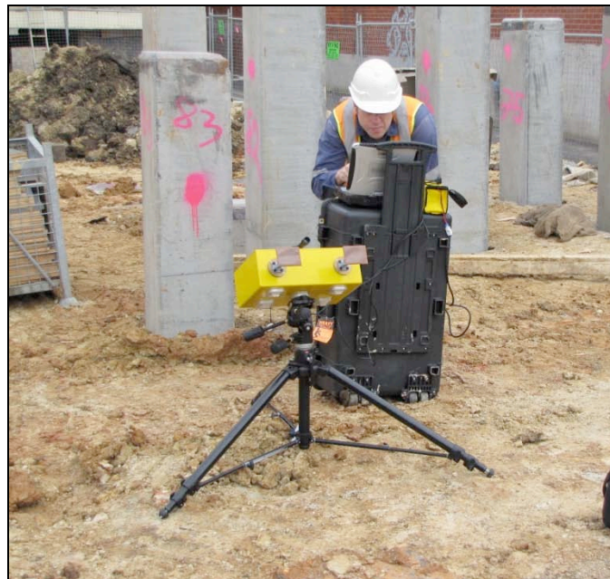
Figure 4: IBIS-S radar set-up and real-time monitoring of deformation.
