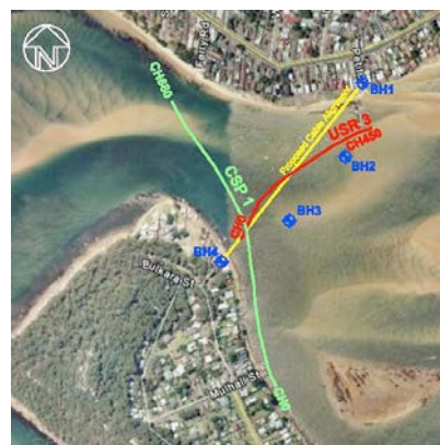
Figure 9 Marine reflection (CSP 1) and underwater seismic refraction (USR 3) trackplots with borehole locations.
