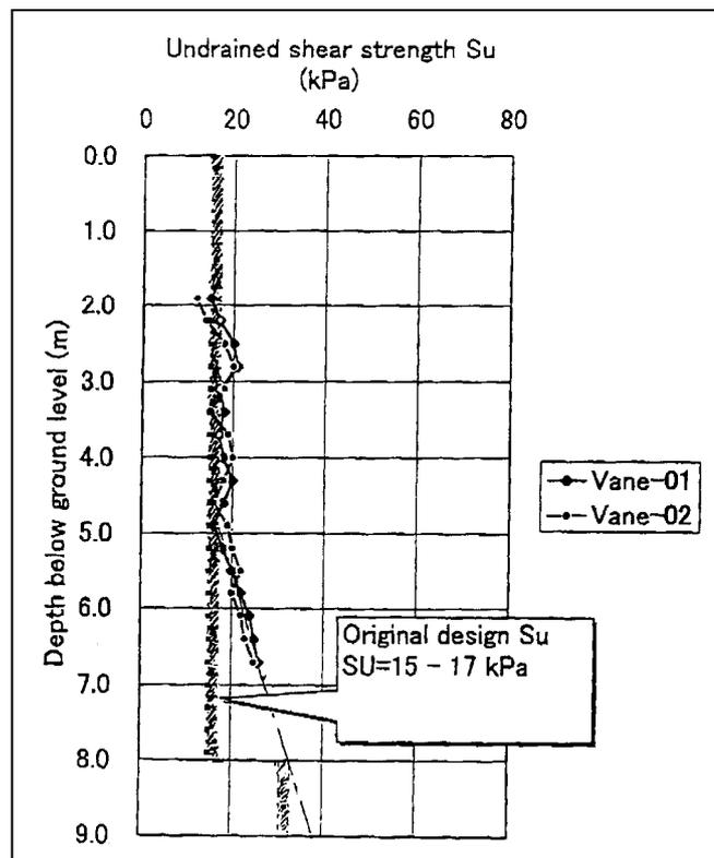
Figure 3: Vane Shear Test Results for Untreated Ground.
