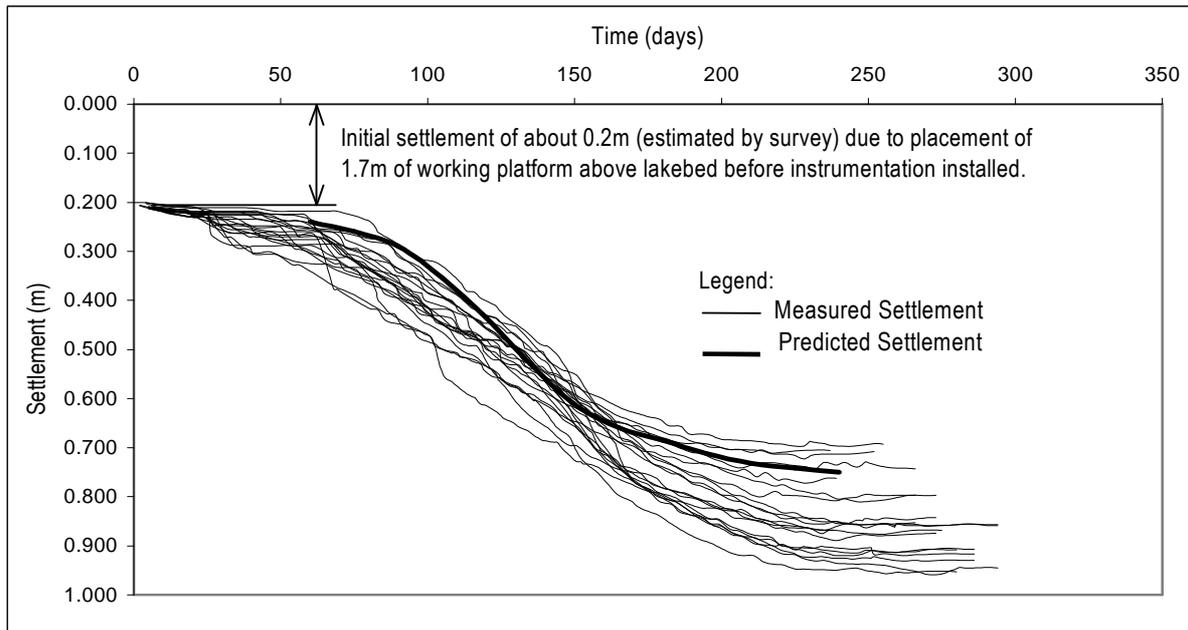
Figure 9: Settlement Monitoring Results (Phase 1).
