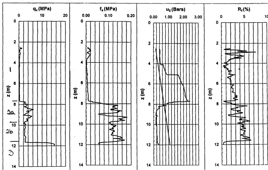
Figure 8: Typical Piezocone Test Result.
