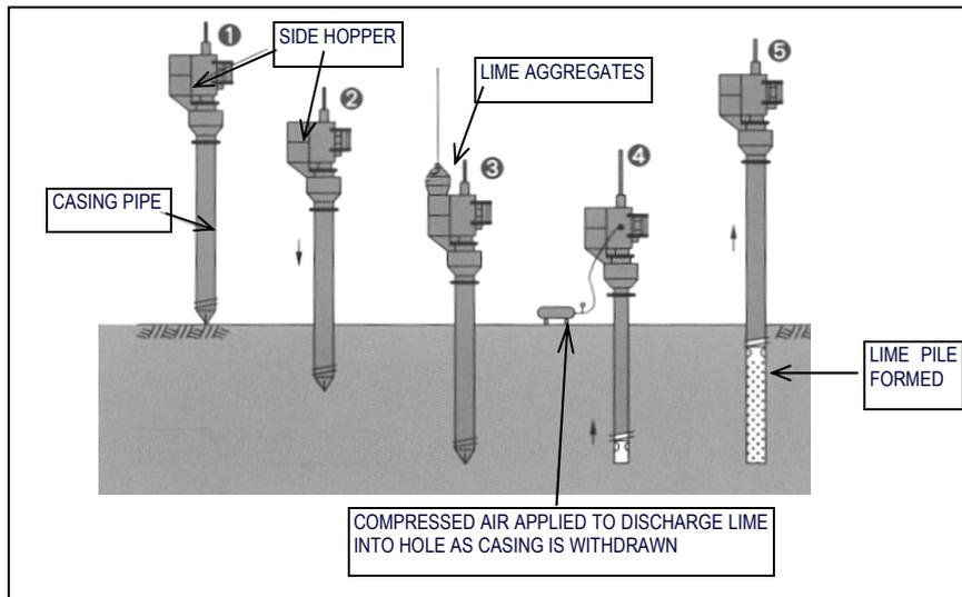
Figure 1: Chemical Lime Pile Installation Process.
