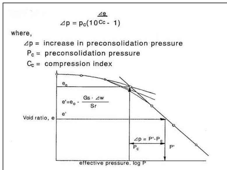
Figure 2: Equivalent Effective Pressure Increase Due to Void Ratio Reduction.
