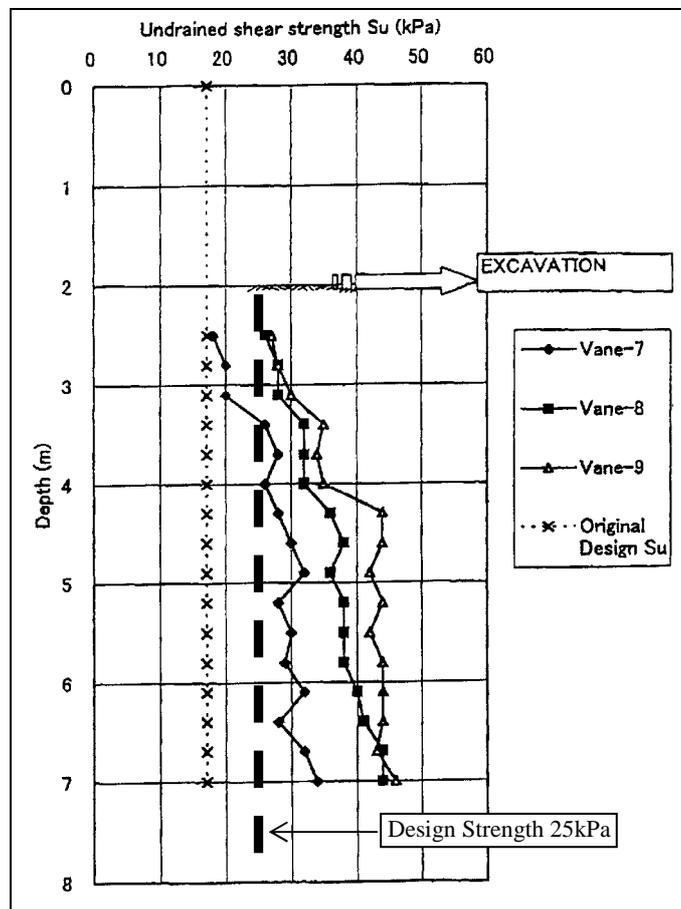
Figure 5: Comparison of Shear Vane Strengths before and after Lime Piling.
