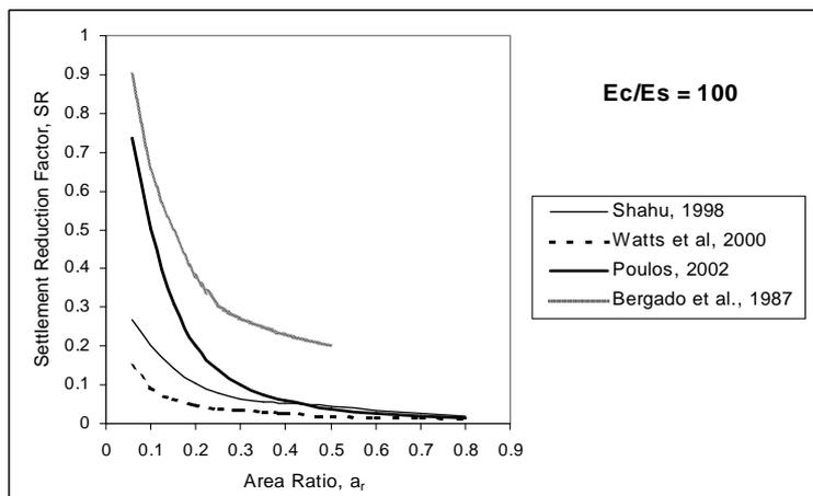
Figure 7(c): Settlement Reduction Ratio for  $E_c/E_s = 100$ .
