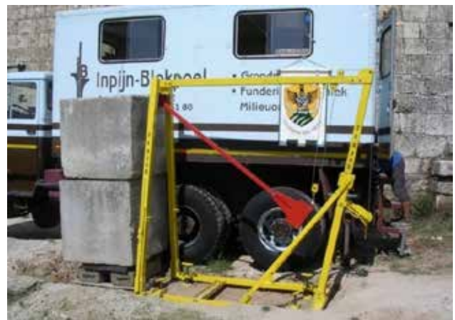
Figure 2. “Enhanced” seismic source (“Tirino Hammer”).
