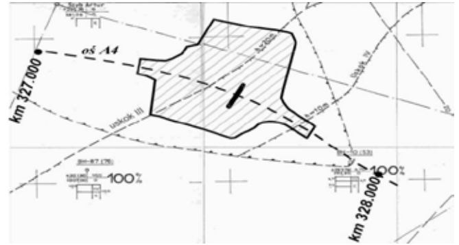
Fig. 3-2. The course of fault III and IV in relation to MOP and A4 motorway (Kotyrba & Kowalski 2009)
