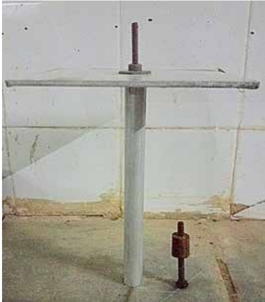
Figure 3. Connection between the pile and the raft.
