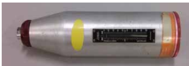
Figure 4. Analogical rebound hammer N type used in lab tests.
