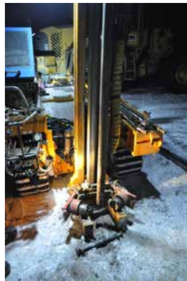
Figure 8. The drilling system with the Atlas Copco core barrel set-up for sampling
