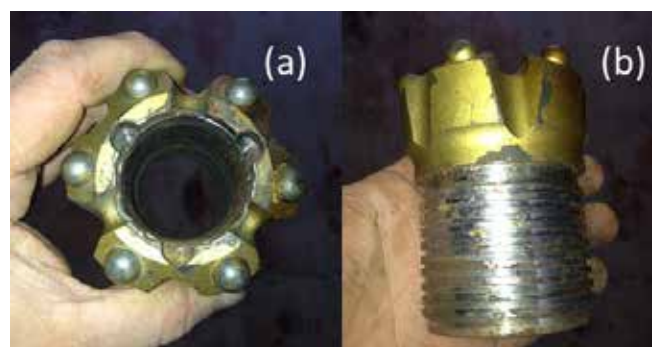
Figure 6. Moraine percussion sample drill bit (a) top view (b) side view
