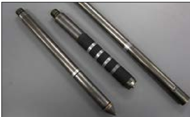
Figure 1: RCPT-u probe (Geotech).
