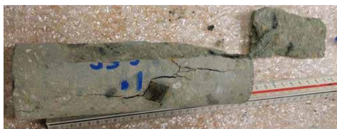
Figure 5. Failed Core Sample
