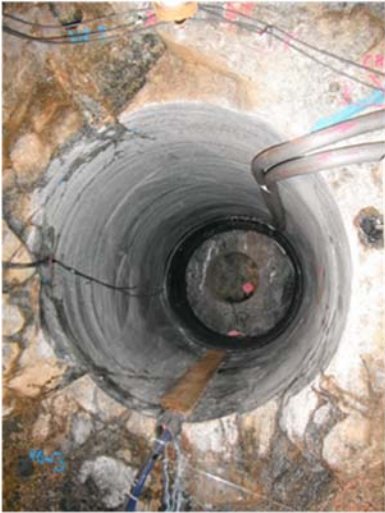
Figure 2. The heating borehole with the heating water pipe
