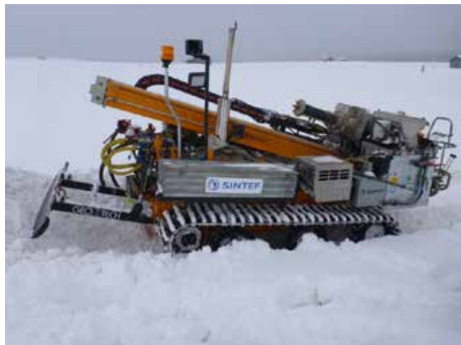
Figure 3. Geotech 504 drilling rig for Arctic condition
