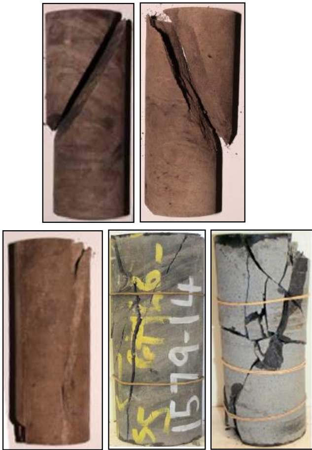
Figure 1. Examples of failure modes of laboratory intact rock testing: shear along defect, shear through intact rock, axial splitting, conical or hour glassing and multiple cracking.
