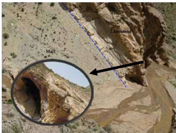
Figure 1. Limestone outcropping on the axis of Lajamgir Dam (large dissolved karst caves)
