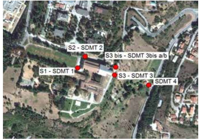
Figure 1. Location of boreholes and V_S measurements by SDMT (in backfilled boreholes and in virgin soil).
