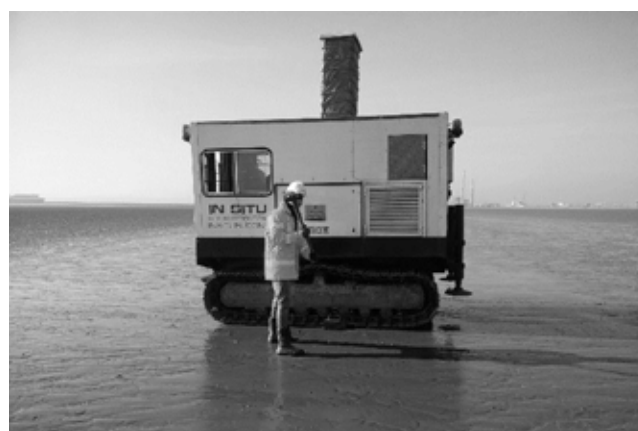
Figure 3. Performing SCPTU test on Bull Island
