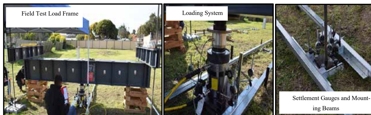
Figure 2. Field testing of Surefoot
