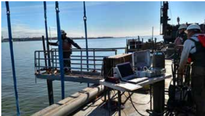
Figure 5: Typical shear wave set-up for SDMT
