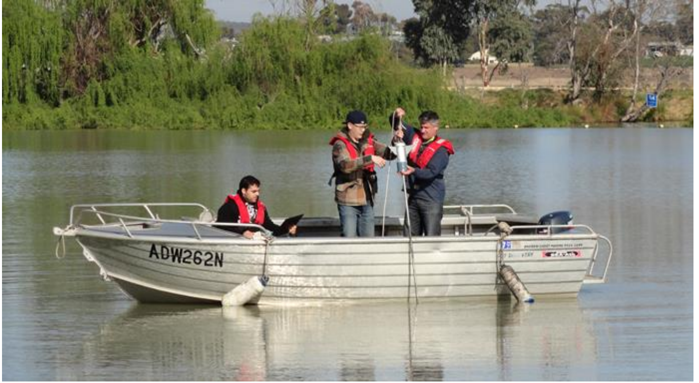
Figure 2. Deployment of the Free Falling Penetrometer
