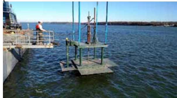
Figure 1. Lowering the seafloor direct push system into the river with a large crane
