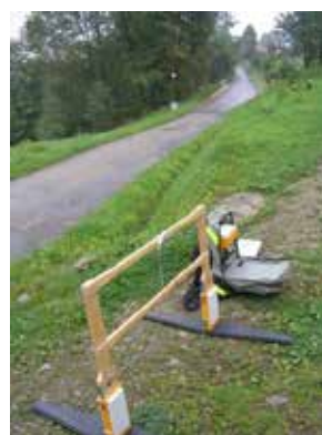
Figure 2. GPR, 100 MHz unshielded antennas, landslide No 21
