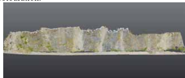
Figure 2. Coloured point cloud of an historic excavated face in a china clay pit
