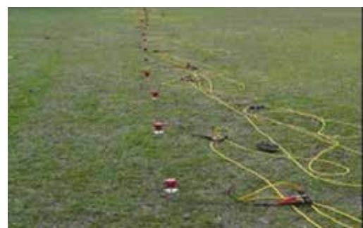
Figure 3. Linear array of geophones
