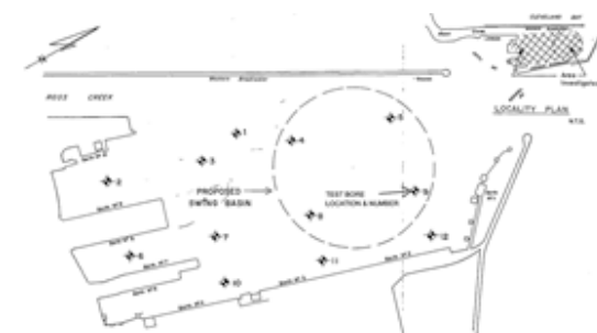
Figure 3. Inner harbor bore holes plan (Douglas Partner 1992)
