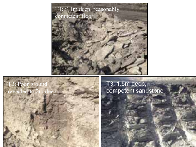
Figure 3. Pit floor conditions revealed from trenches. Very poor ground shown in the trench T2.
