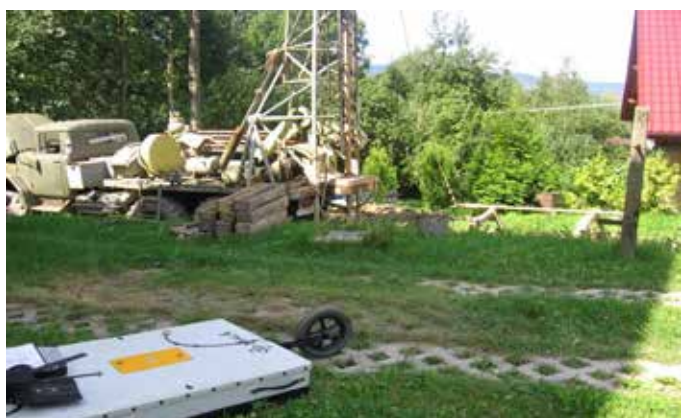
Figure 4. GPR scanning close to the borehole, landslide No 23
