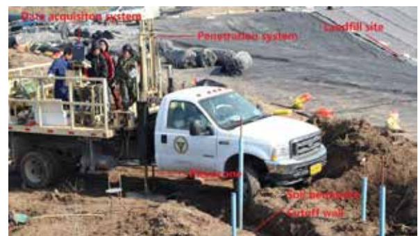
Figure 2. The in-situ piezocone penetration test in cutoff wall of landfill site
