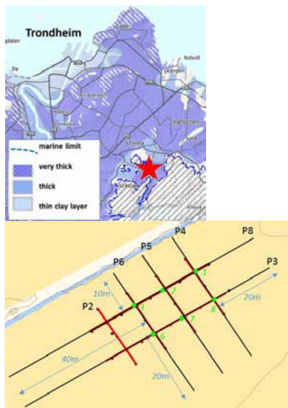
Figure 1. Upper: Dragvoll site. Lower: The ERT survey before salt-well installation is illustrated in thick red lines while the two later surveys are in thin black lines. The salt wells are numbered in green (1, 2, 3, 6, 7, and 8).
