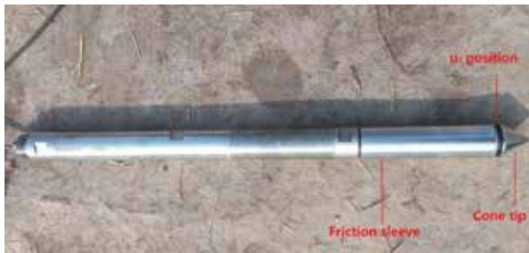
Figure 3. The piezocone used in this test site
