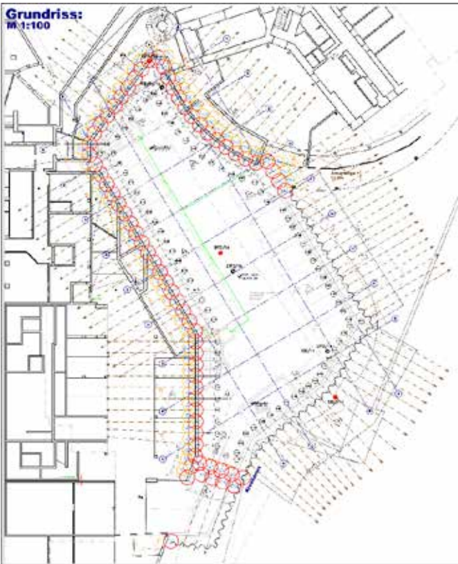
Figure 6. Layout of Jet-Grouting and Pile Wall
